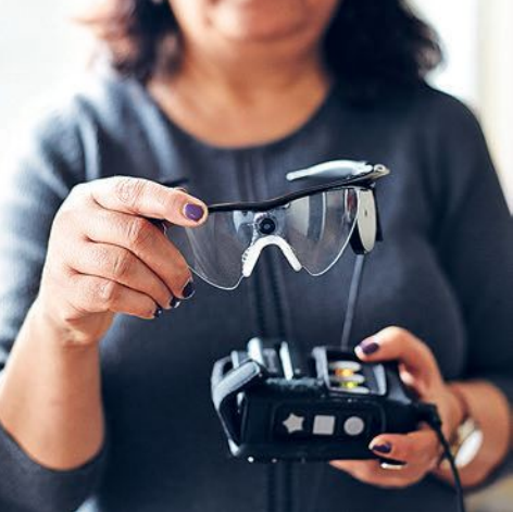
The Argus sends data from camera-equipped glasses to a retinal implant.
